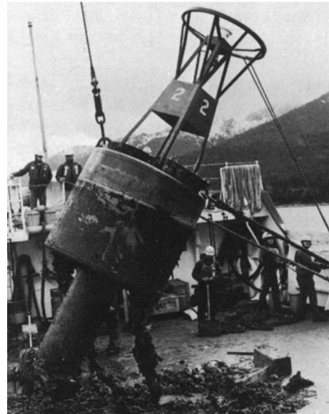
Figure 509. Buoy showing counterweight.
