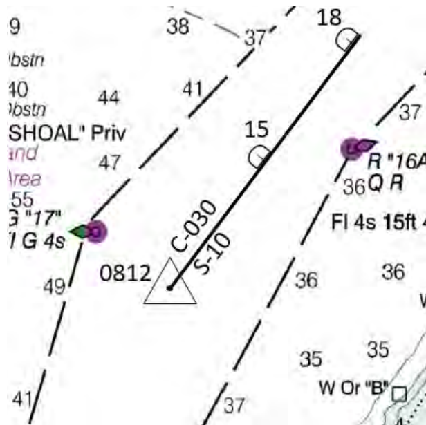
Figure 4a. A radar fix with DRs clearly labeled.
