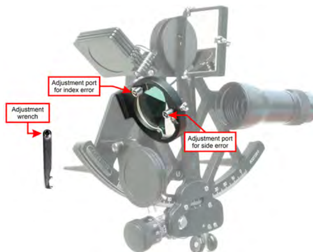
Figure 1511g. Adjustment port on the horizon glass and an adjustment wrench.
