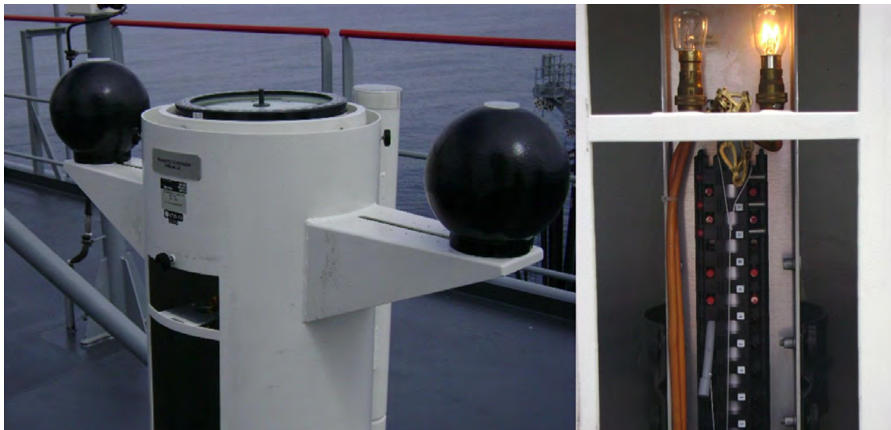
Figure 918c. Modern magnetic compass binnacle showing Flinder Bar tube, Quadrantal Spheres and the fore-and-aft/athwartships magnets.
