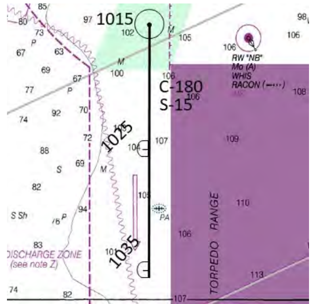
Figure 4b. A visual fix with DRs clearly labeled.
