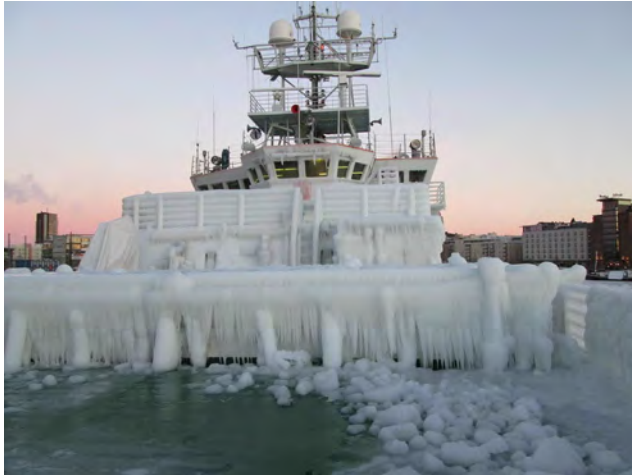
Figure 4204a. Ice accumulation on deck can cause significant problems with stability of small ships. Freezing spray conditions should be avoided when possible. Image courtesy of Lars Anderson, SMHI.
