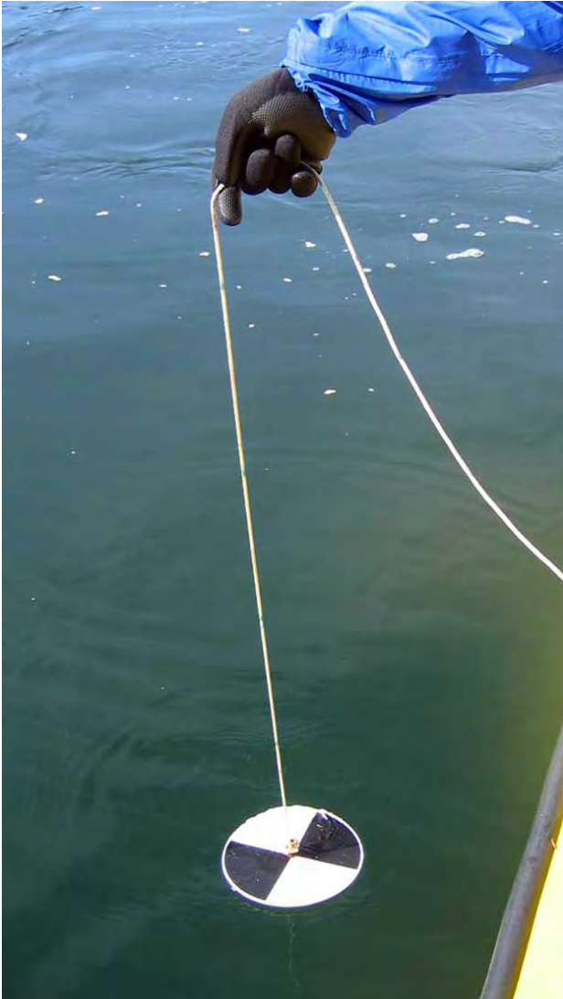
Figure 3515. A Secchi disk is used to measure sunlight penetration through the water.
