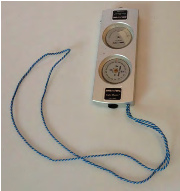
Figure 1721. Combined compass/inclinometer with internal lighting and automatic leveling.
