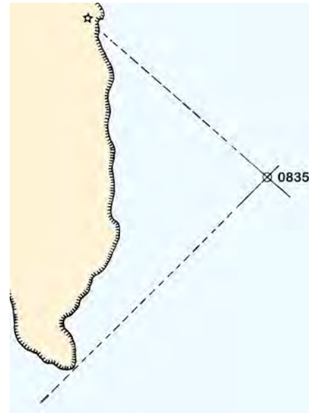
Figure 1111a. A fix by two bearing lines.
