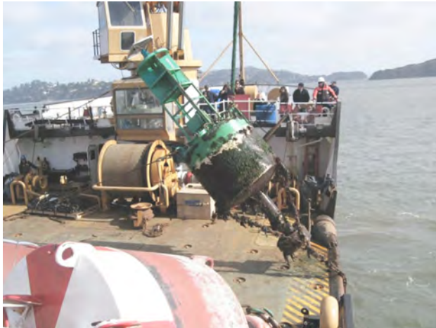
Figure 801a. Buoy with counterweight showing.
