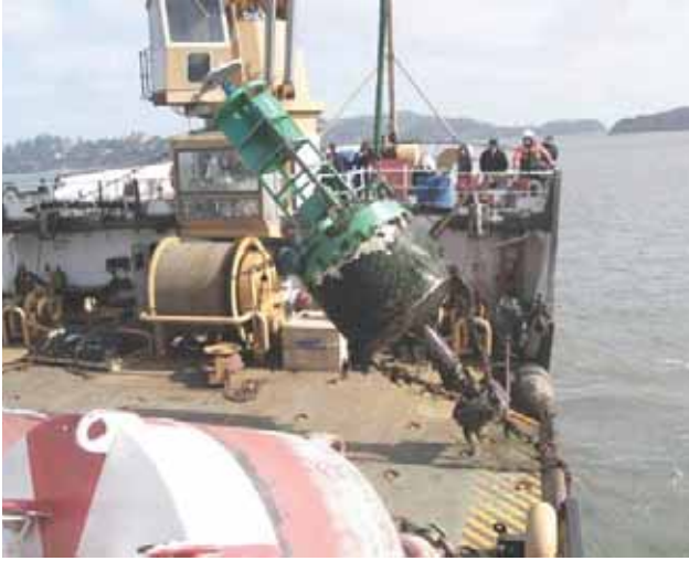
Figure 701a. Buoy with counterweight showing.
