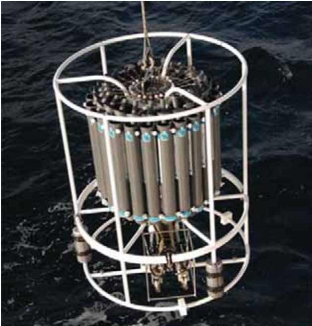
Figure 3402. CTD Rosette is lowered to measure the salinity, temperature, depth and concentration of particles in the water column. Image courtesy of NOAA.
