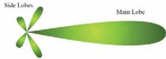
Figure 2306a. Freespace radiation pattern.
