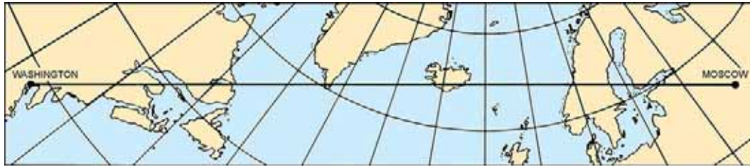
Figure 409c. An oblique Mercator map based upon a cylinder tangent along the great circle through Washington and Moscow. The map includes an area 500 miles on each side of the great circle. The limits of this map are indicated on the Mercator map of Figure 410.
