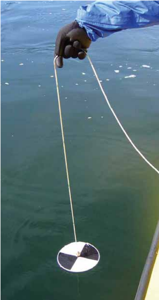
Figure 3415a. A Secchi disk is used to measure sunlight penetration through the water.
