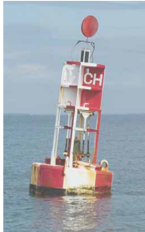
Figure 733b. Safe water buoy.
