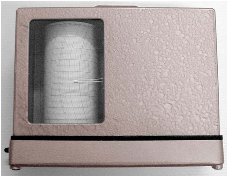
Figure 4003. A marine barograph.
