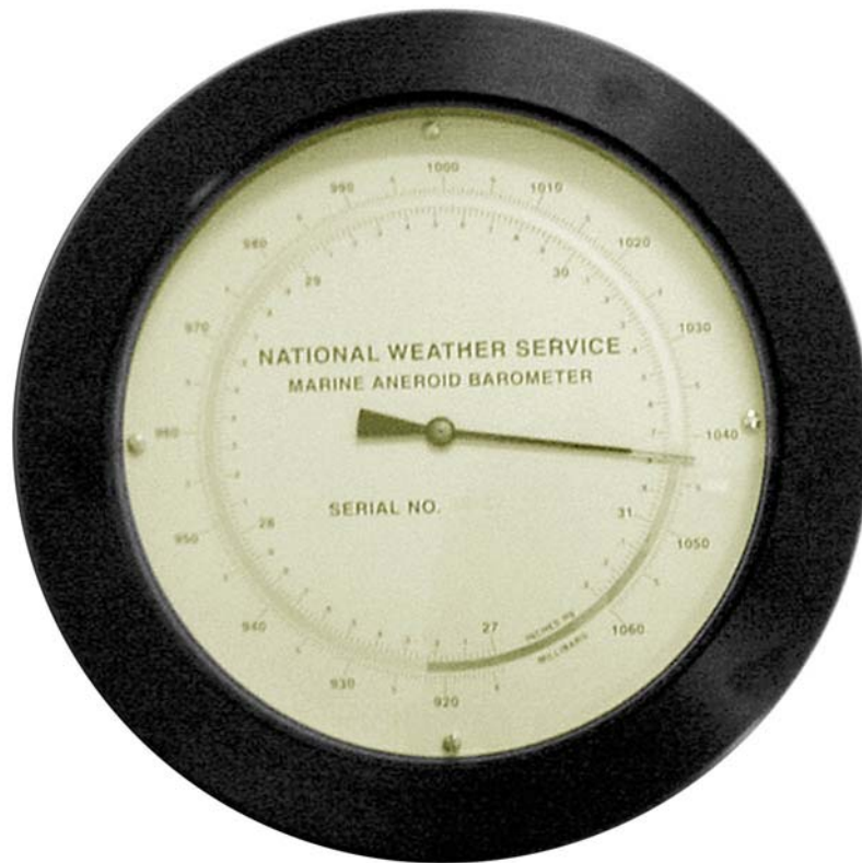
Figure 4002a. An aneroid barometer.
