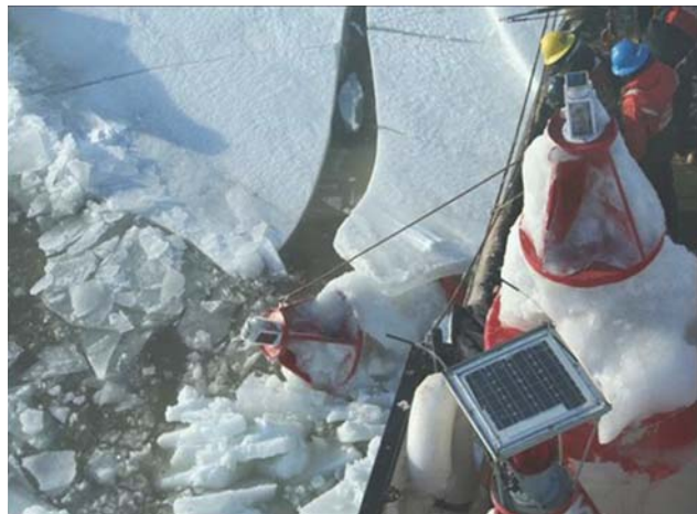
Figure 706. USCG recovering ice damaged buoys.
