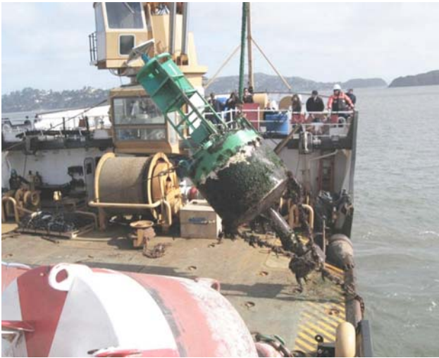
Figure 701a. Buoy with counterweight showing.
