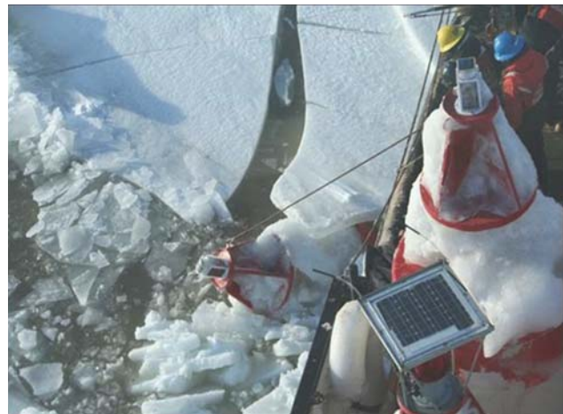
Figure 706. USCG recovering ice damaged buoys.
