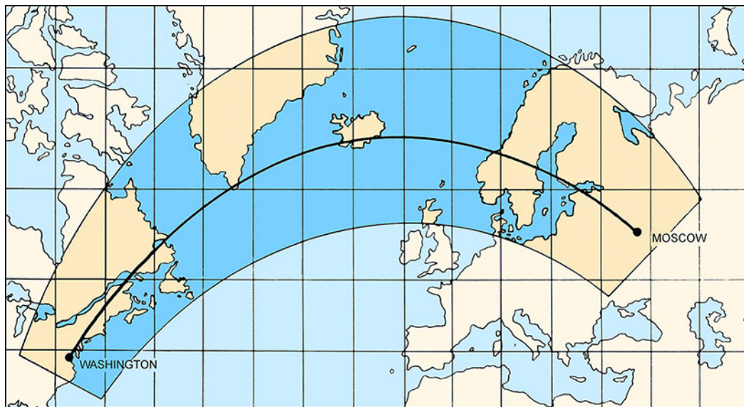
Figure 410. The great circle between Washington and Moscow as it appears on a Mercator map.
