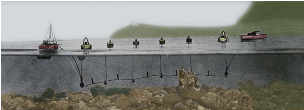
Figure 305. Conducting a wire drag. Image courtesy of NOAA.
