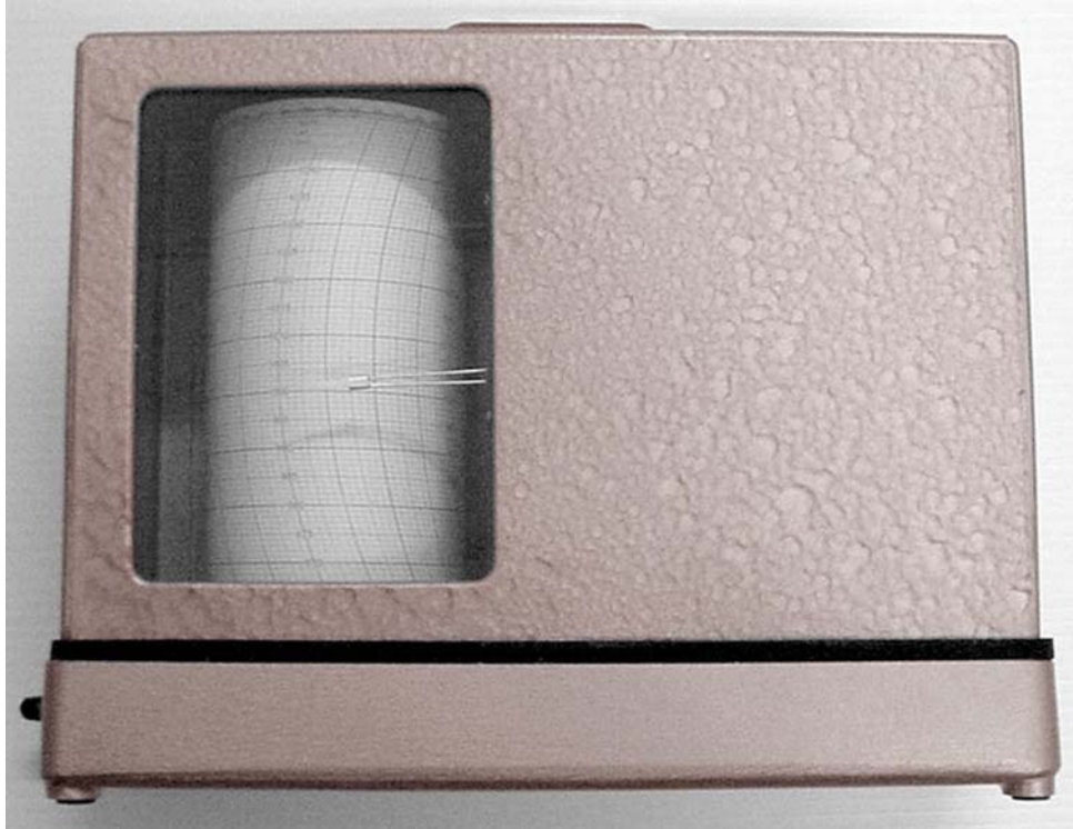
Figure 4003. A marine barograph.
