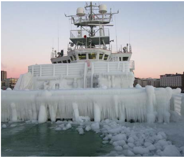
Figure 4104a. Ice accumulation on deck can cause significant problems with stability of small ships. Freezing spray conditions should be avoided when possible. Image courtesy of Lars Anderson, SMHI.
