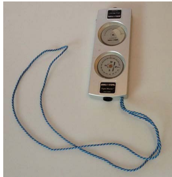
Figure 1619. Combined compass/inclinometer with internal lighting and automatic leveling.
