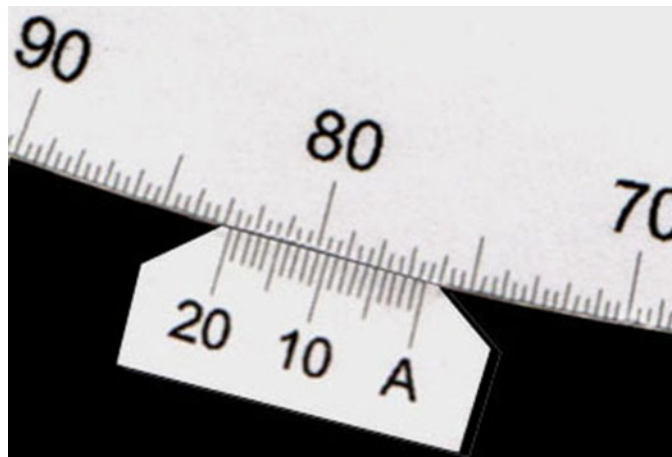
Figure 1408b. Vernier sextant set at 76^{\circ} 26' 00'' . Image courtesy of Omar F. Reis.
