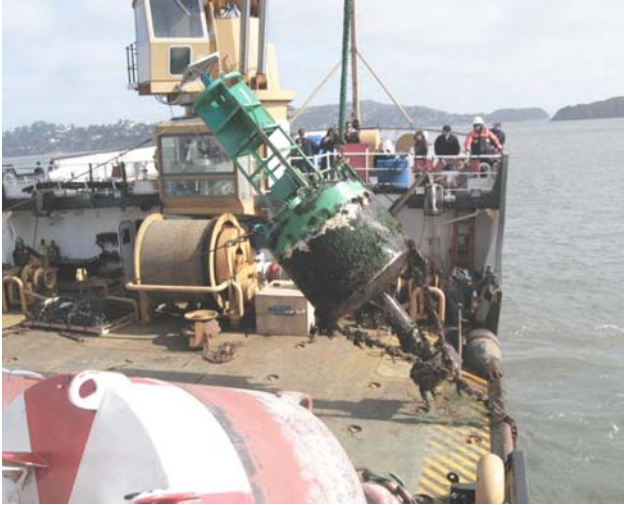
Figure 701a. Buoy with counterweight showing.
