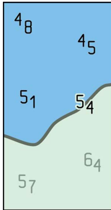
Figure 521f. This image shows depth labels (with a light “halo” to set them apart) and soundings both deeper and shallower than the safety depth. Image courtesy of NOAA.
